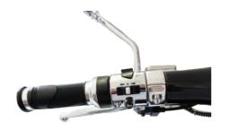
On the left hand side are the buttons for **the indicators** and the hon. You are able to switch between full- and dimmed beam.
