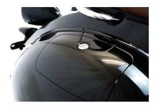
On the right of the e-scooter is a **lockable com- partment.** Is its perfect for stowing things like a charger, keys, a mobile phone or a wallet.
